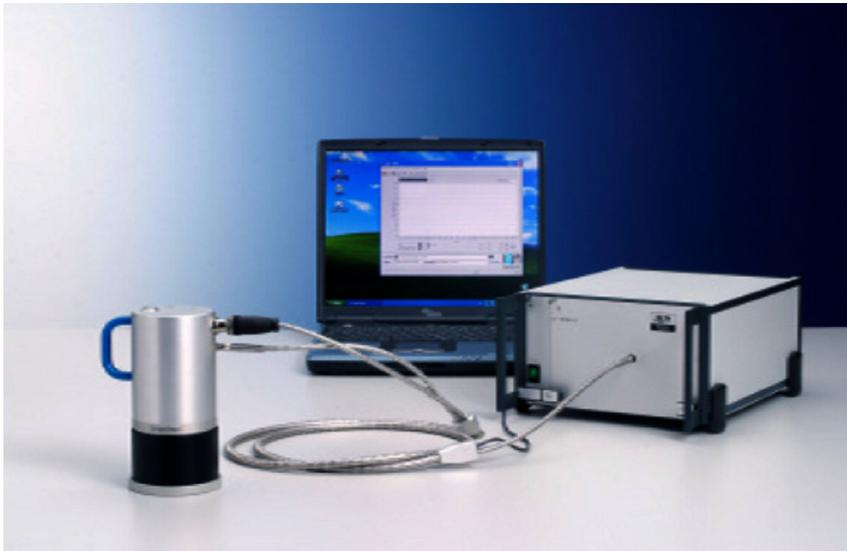
**Sample cells like reflection measuring heads or others are available and connected by fiber optics.**
