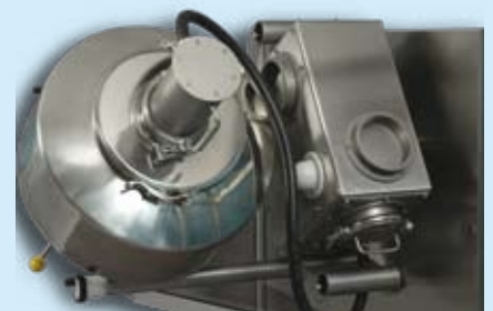
Fig. 3: Installation of an IRIS-7 with spectrometer mounted to a blend system
