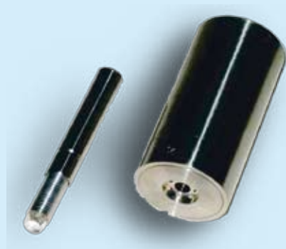
Fig. 1: Measurement head with light source for reflection spectroscopy.
