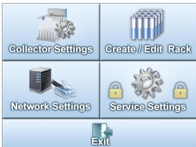
The menu item "System Settings" is divided into four areas - the area for the fraction collector settings, the area for the rack configuration, the area for network configuration and a service area. You enter the areas by tapping on the respective items. The "Exit" item will bring you back to the main menu.
