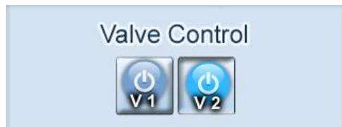
By tapping the respective button, the corresponding valve is activated or deactivated.
