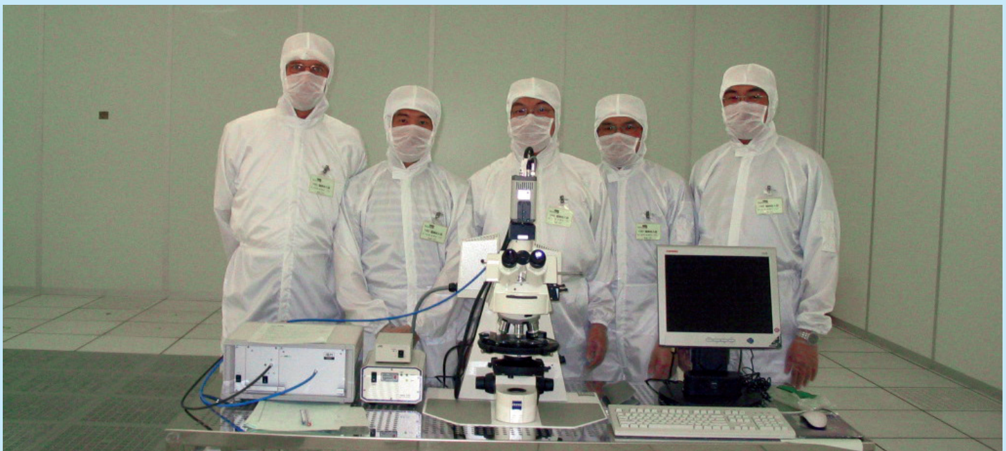
MSP 400 in a cleanroom, used in quality control of TFT displays
